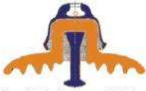
Figure 1 Section view of a porcelain insulator
