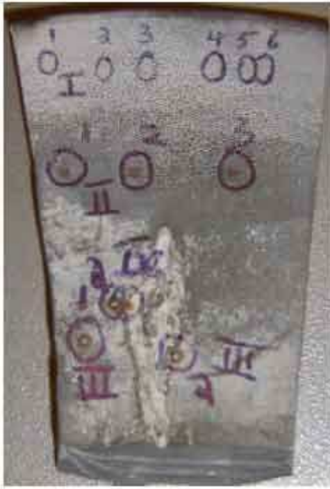
Fig 10: Laser induced changes along the first shed indicated by the circles numbered 1-6
